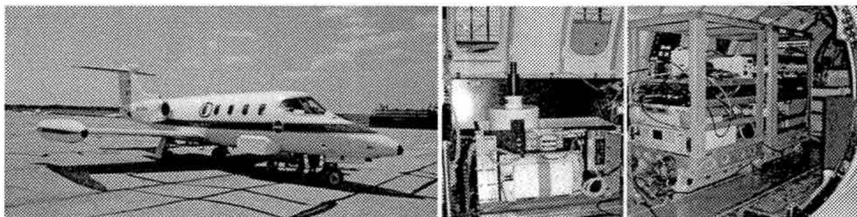
Figure 1- Left - NASA Glenn Lear-25 aircraft. The nadir window assembly is just below the NASA logo. Photographs of the lidar installed on the aircraft showing the sensor head assembly ( Middle ) and the dual aircraft racks ( Right ).
