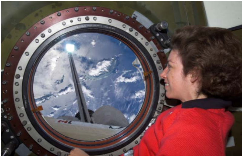
US Laboratory Window 50-cm diameter Telescope-quality optical glass NADIR view
