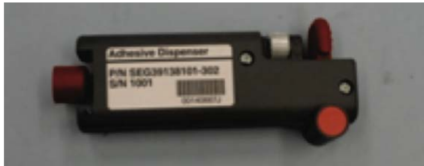
Figure 7.1-6. RTV Syringe Dispenser
