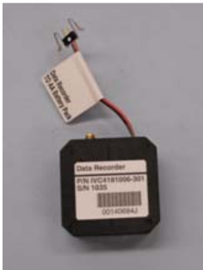
Figure 7.1-2. RSU Transceiver Module Modified for an External Battery (top right) and External Antenna Connection (top left)
