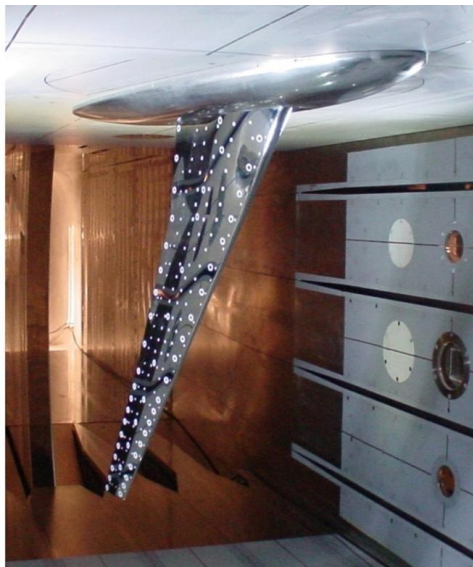
Figure 8. HIRENASD installed in ETW.
