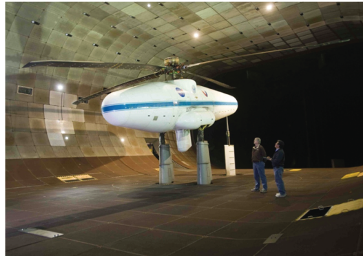
Figure 1: Full-scale UH-60A rotor installed on the Large Rotor Test Apparatus in the NFAC 40- by 80- ft wind tunnel.
