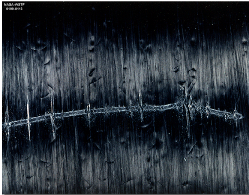
Small cylinder, significant scratch, transverse to winding direction
