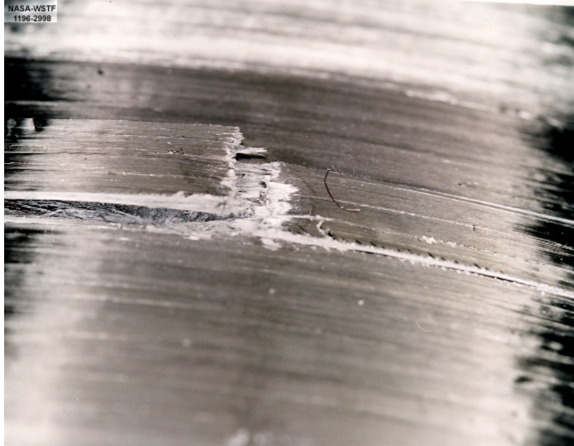
Large Cylinder, 4500 Hydraulic, 35 ft-lb Impact, 0.5 in. Tup, Oblique View in Direct Light
