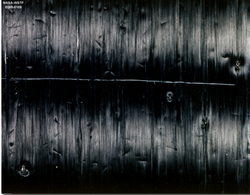
Small cylinder, cut, transverse to winding direction
