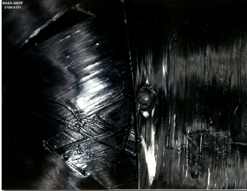
4 x 9 in. cylinder, broken tow
