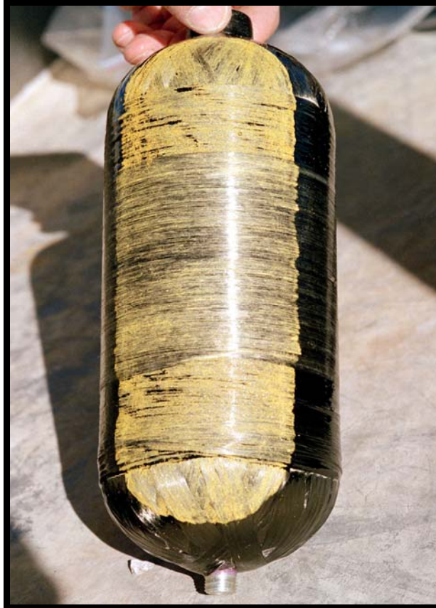
SCI Subscale Vessel after N 2 O 4 Exposure
