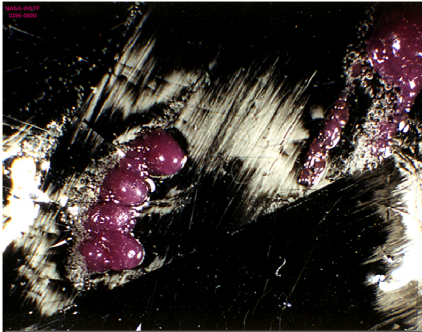
4 x 9 in. cylinder, excess bonding agent, magnified view
