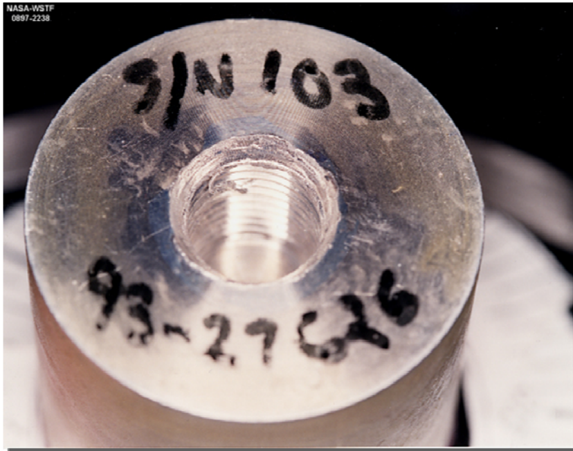
Inlet thread damage
