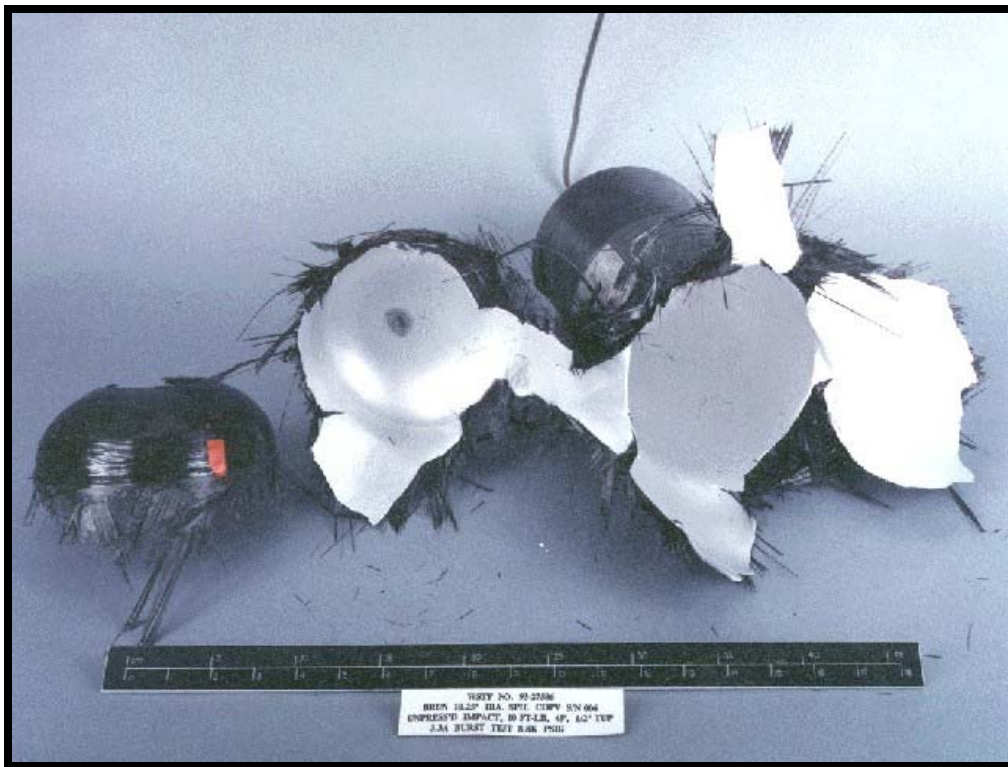
Small Cylinder Postimpact Burst
