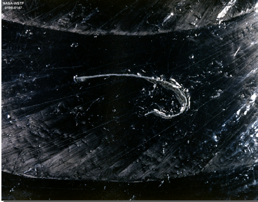
4 x 9 in. cylinder, entrained fiber
