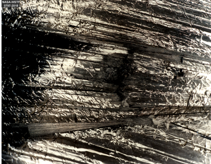
Large Sphere, 4725 psi Pneumatic, 100 ft-lb, 0.5 in. Tup
