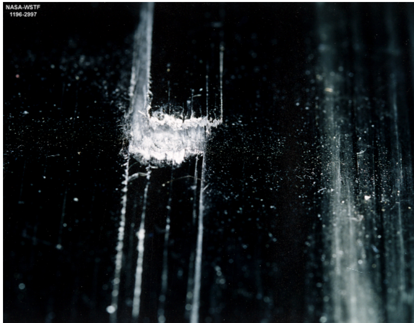
Large Cylinder, 4500 Hydraulic, 35 ft-lb Impact, 0.5 in. Tup, Oblique Lighting
