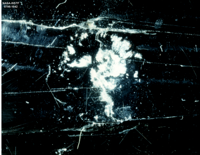
Small Sphere, 6000 psi Hydraulic, 35 ft-lb Impact
