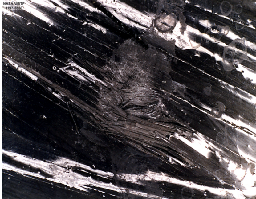
Large Sphere, 4500 psi Hydraulic, 15 ft-lb Impact, 0.5 in. Tup
