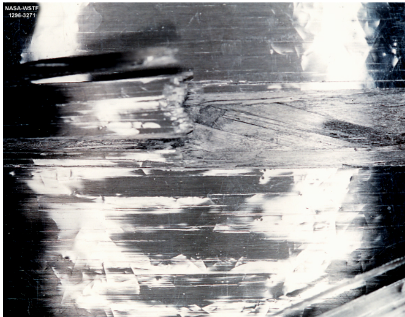
Large Cylinder, 4500 Hydraulic, 35 ft-lb Impact, 0.5 in. Tup
