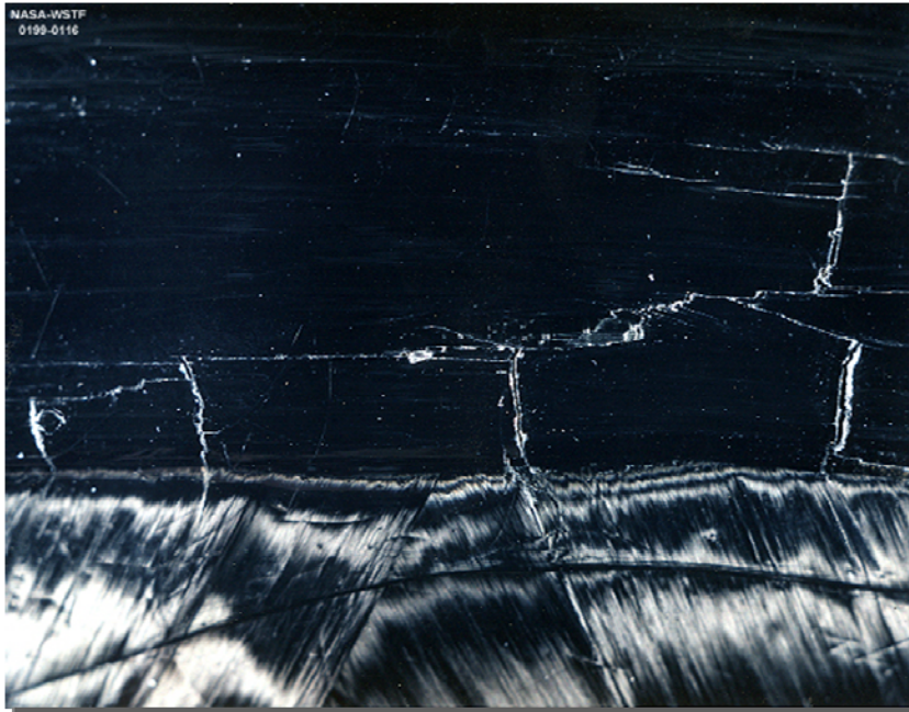
Small cylinder, manufacturing defect, nonelastic end crack
