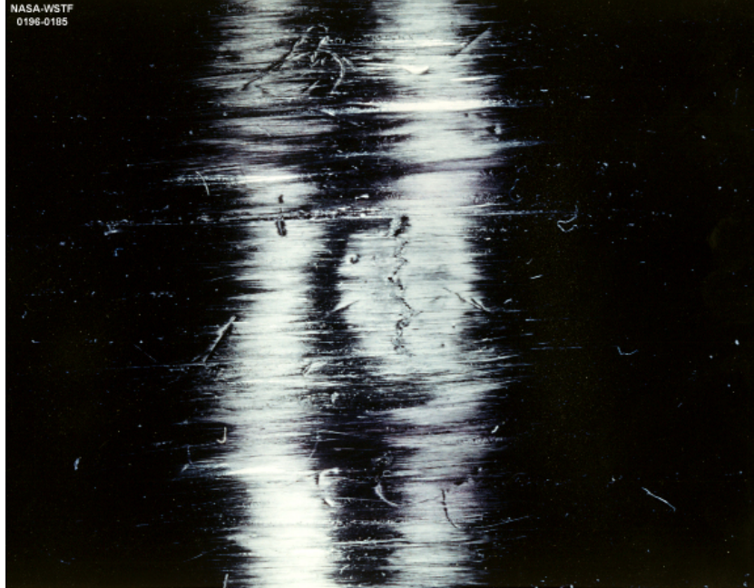
Small Cylinder, 6000 psi Hydraulic, 15 ft-lb Impact, 0.5 in. Tup
