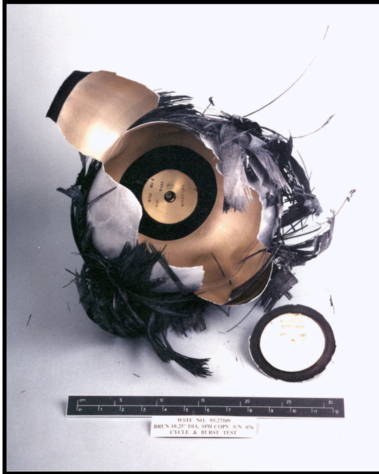
Small Sphere Undamaged Burst
