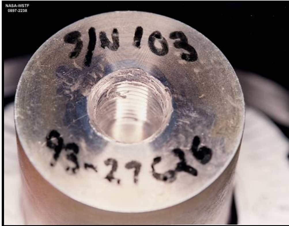
Inlet Thread Damage
