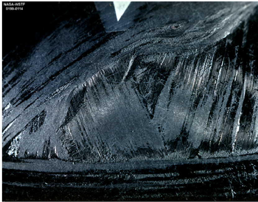
4.6 x 10 in. cylinder, significant abrasion
