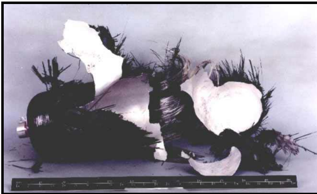
Small Cylinder Undamaged Burst
