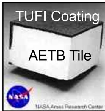
TUFU =Toughened Uni-piece Fibrous Insulation
