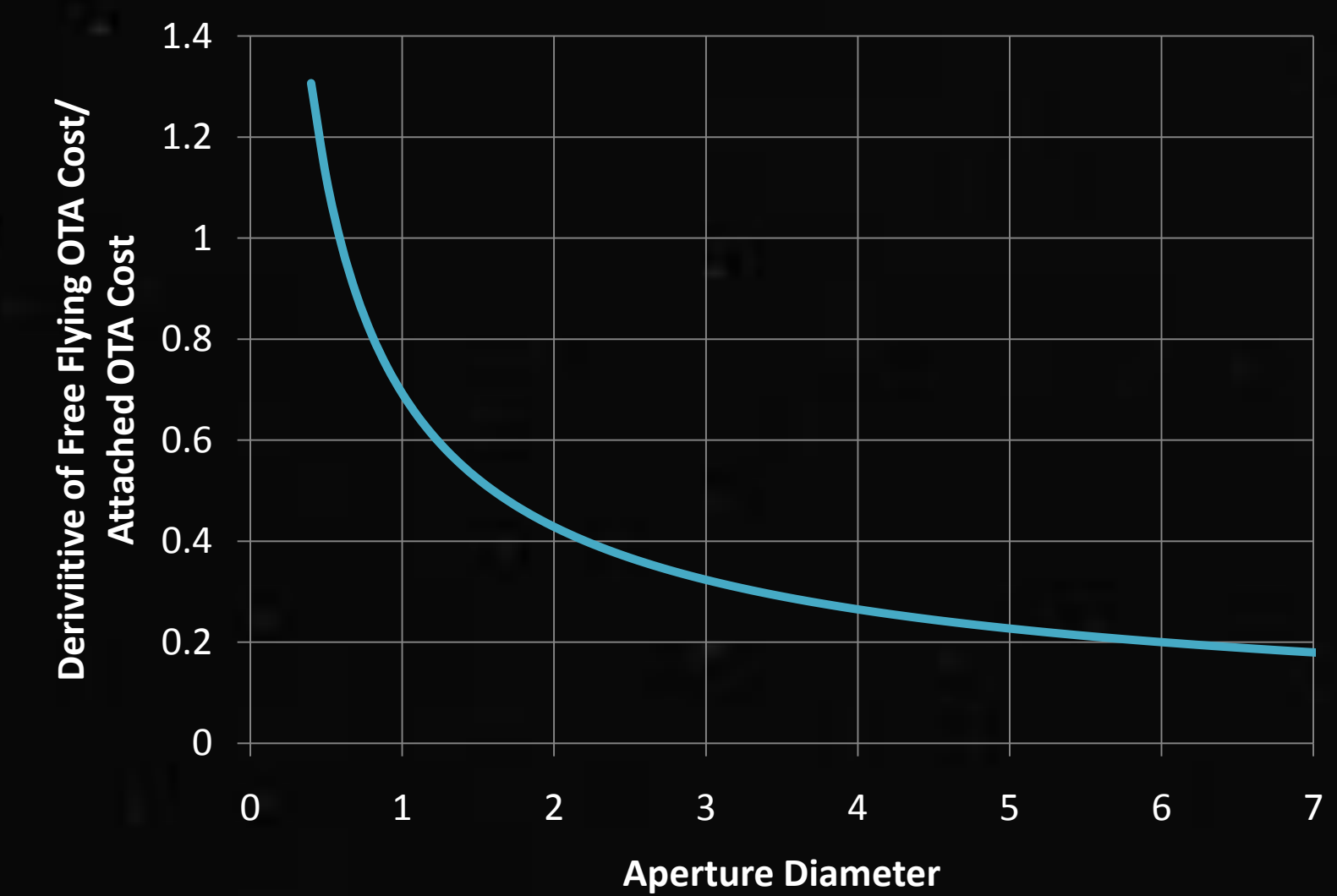
Middle Plot: Demonstrates the ratio of Free Flying OTA Cost to Attached OTA Cost versus diameter. This shows how many more times cost is for free-flying versus attached telescopes. Bottom Plot: Shows the rate of change or slope of the middle plot.
