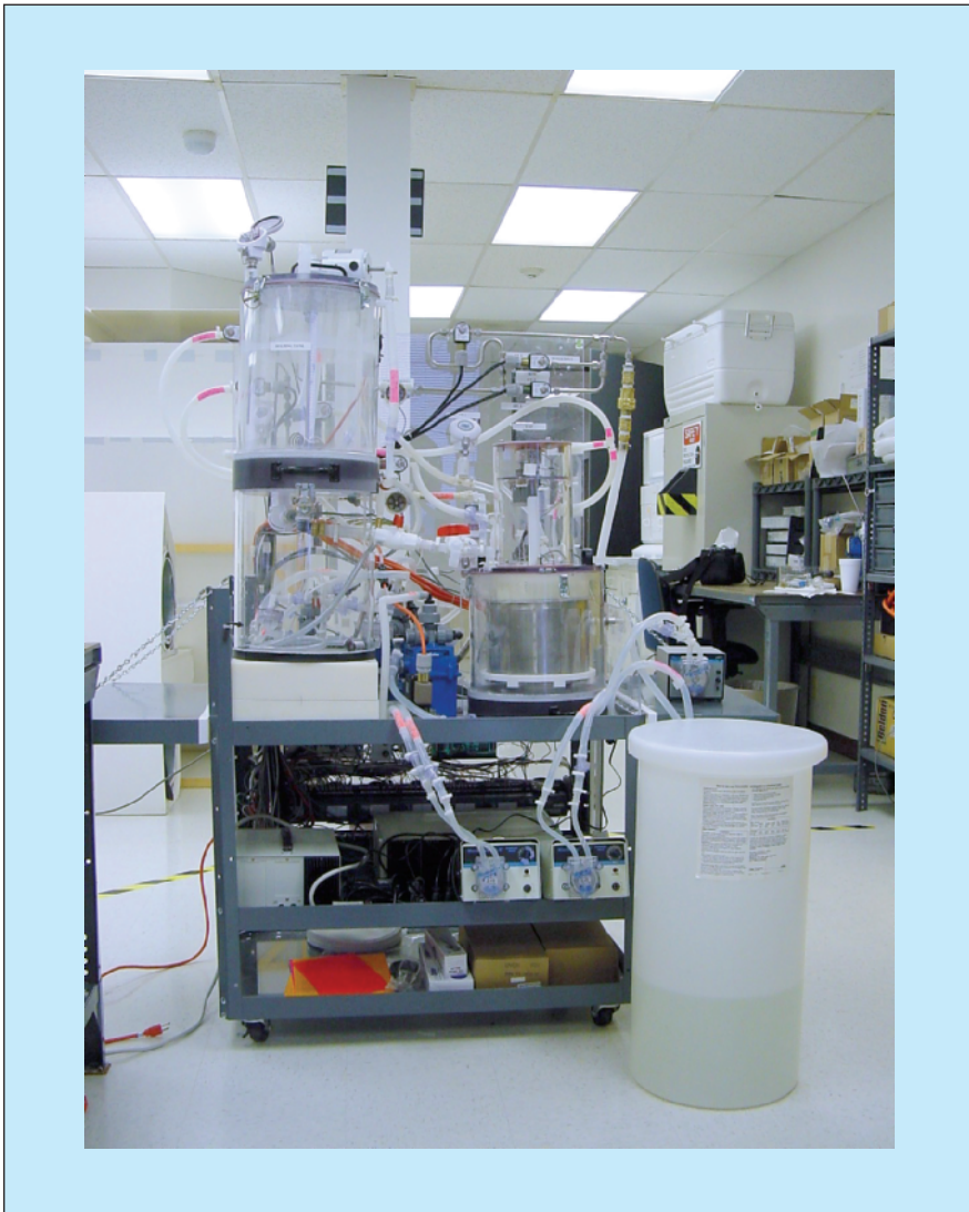
This Laboratory Apparatus is a prototype of scientific, industrial, and household soy-processing systems for processing batches of soy under selectable, reproducible conditions.
