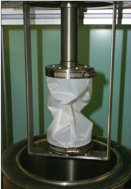
A Flex Testing Apparatus repeatedly twists and compresses a sample of material.
