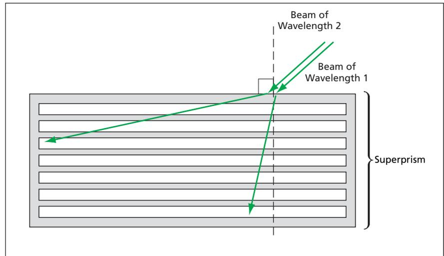
A One-Dimensional Superprism could be fabricated more easily than a three-dimensional superprism. Like a three-dimensional prism, it would exhibit strong wavelength dispersion: two beams of light incident at the same angle and having slightly different wavelengths would be refracted at two widely different angles.
