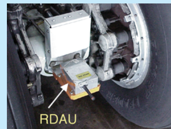
RDAU Mounted on Tow Fitting of Landing Gear
