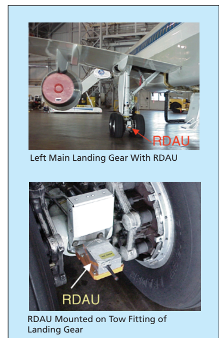
Figure 2. An RDAU Mounted on a Landing Gear was used to perform a rigorous test of the system.
