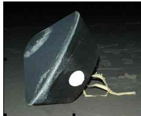
Image of the sample return capsule post flight with PICA as the forebody TPS.
