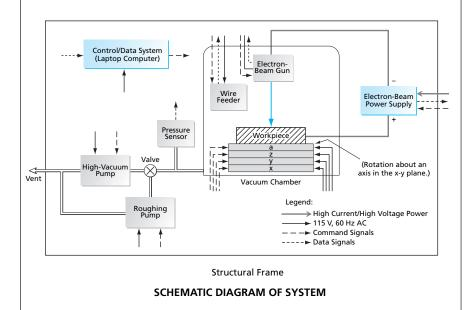
A **Metal Workpiece Will Be Formed** by using an electron beam to melt feed wire over a substrate that will be moved by a four-axis positioning subsystem.
