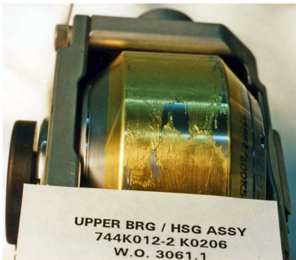
Figure 11.—Upper roller from starboard SARJ, showing peeling of the gold plating prior to assembly into trundle.
