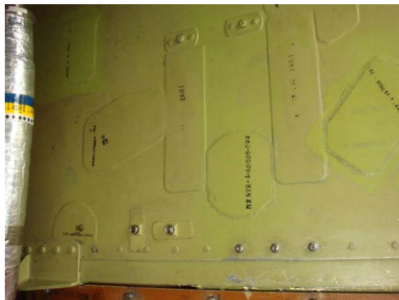
Figure 5-4. Typical Avionics Bay Honeycomb Panel Damages.
