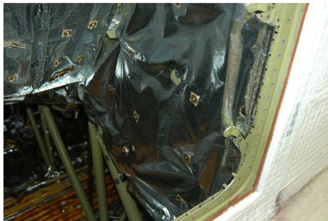
Figure 5-2. Main Ingress/ Egress into the Space Shuttle Mid-Fuselage Compartment. Highly sensitive thin Boron/ Aluminum Struts line ingress/ egress route.
