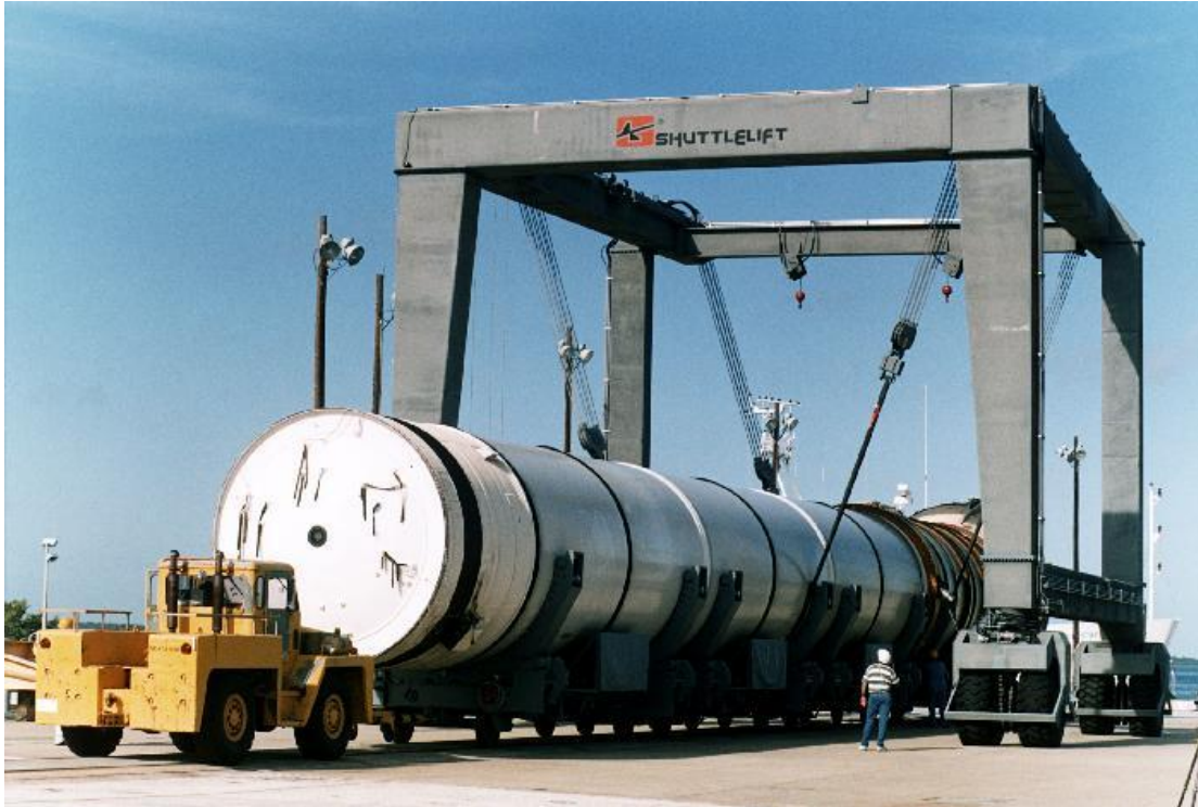
Figure B.2-32 Recovered SRB Being Placed on Dollies at Hangar AF
