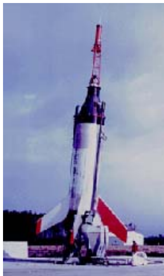
Figure B.4-1 Capsule Escape Rocket Testing
