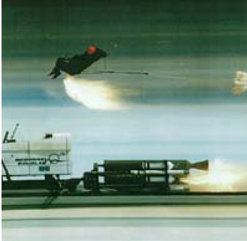
Figure B.13-7 Ejection Seat Testing
