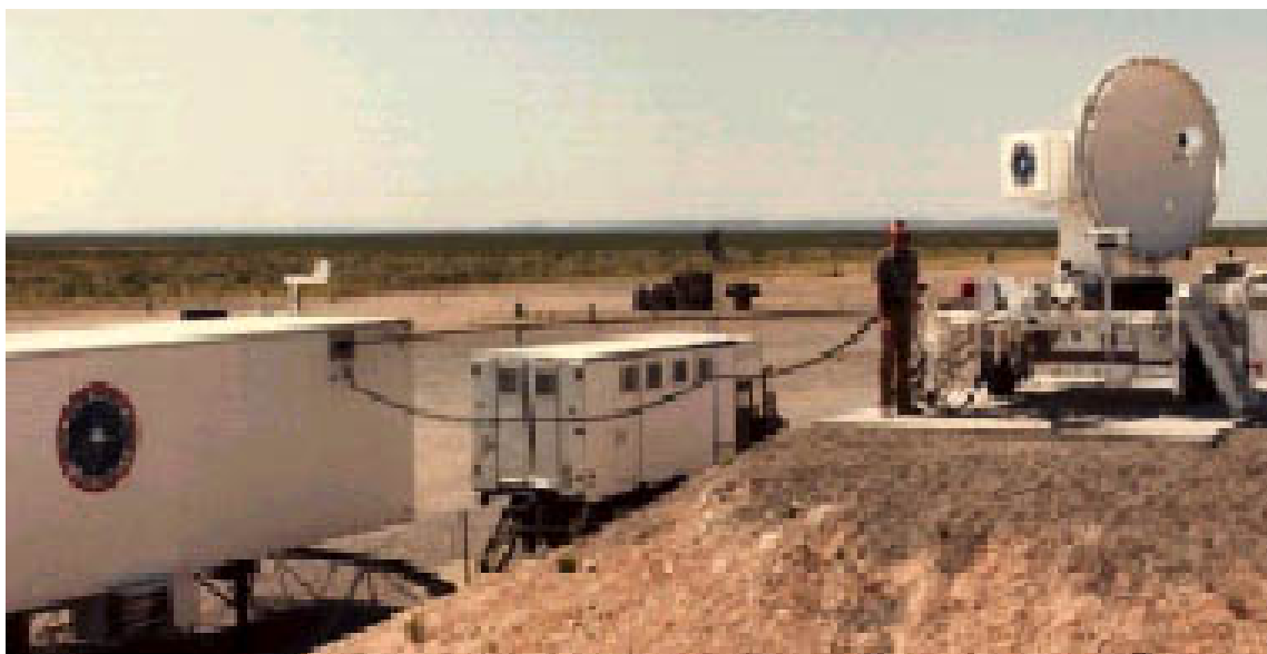
Figure B.7-22 Miss Distance Indicating Radar
