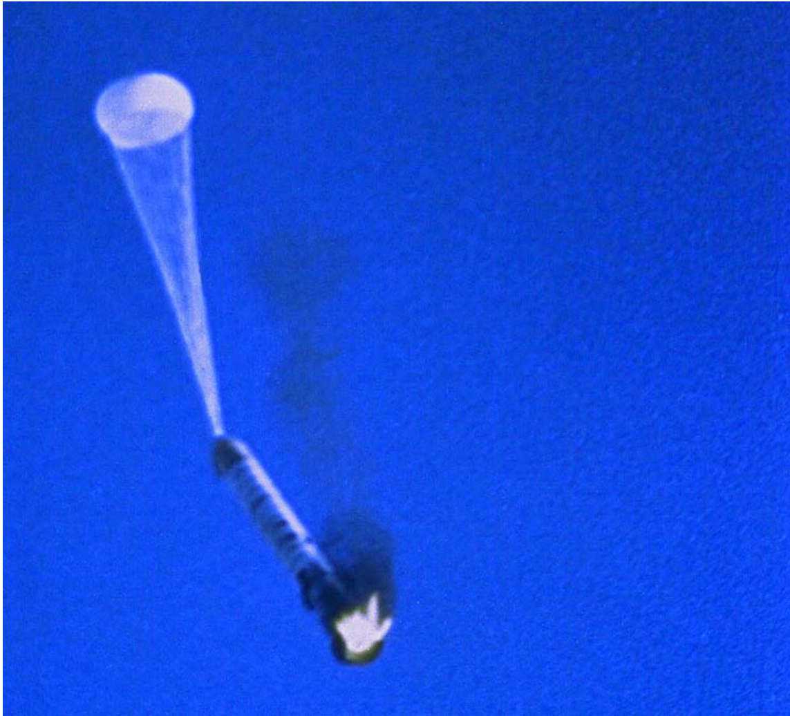
Figure B.2-44 SRB With Drogue Chute During Descent
