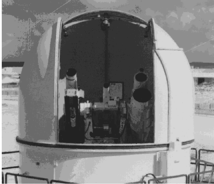
Figure B.5-13 RTS Optical Tracking Camera
