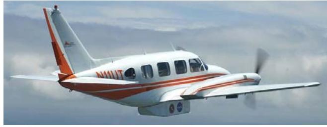
Fig. 2. MAPIR enclosed in fairings beneath a Piper Navajo.
