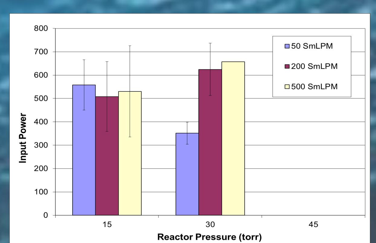
Testing indicated that CO<sub>2</sub> plasma was more easily ignited at lower pressures. It was not possible to ignite the CO<sub>2</sub> plasma at 45 torr.
