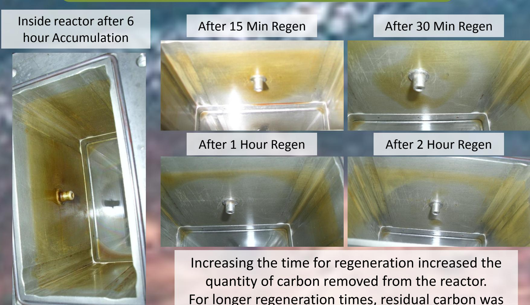
Increasing the time for regeneration increased the quantity of carbon removed from the reactor. For longer regeneration times, residual carbon was more easily removed by mechanical means.
