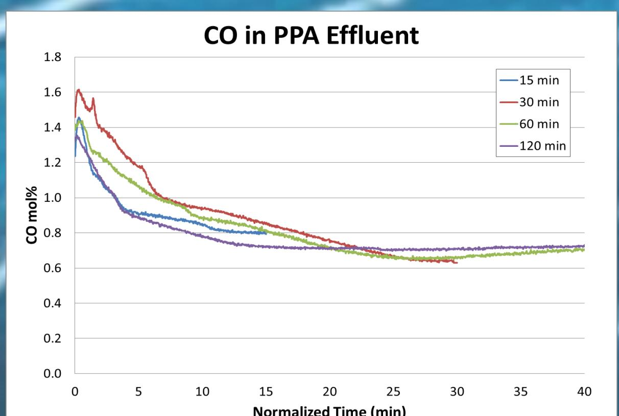
Carbon monoxide was produced in similar quantities and for similar lengths of time for each trial.
