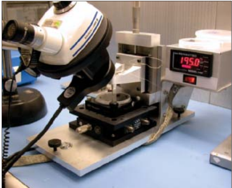
This Microchip-Bonding Apparatus produces better, more repeatable microchip/substrate indium bump bonds than did a prior apparatus.
