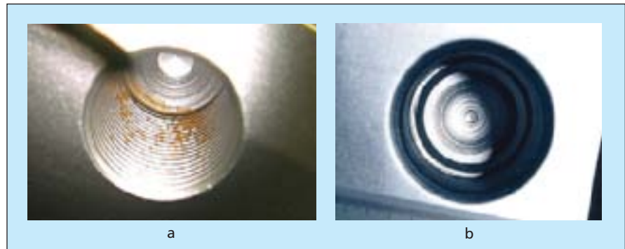
In a Blind Hole in a D6AC Steel Specimen washed with deionized water, corrosion products can be seen on the thread (a). There is no visible sign of corrosion in a similar specimen rinsed with the corrosion-inhibited solution (b).
