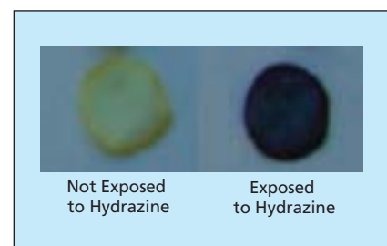
A Porous Cellulose Disk Loaded With \text{KAuCl}_4 changes color upon exposure to hydrazine.
