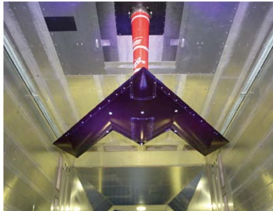
Figure 1 SACCON low-speed wind tunnel model inverted in the dynamic Model Positioning Mechanism in the closed test section of the Low-Speed Wind Tunnel Braunschweig (DNW-NWB).
