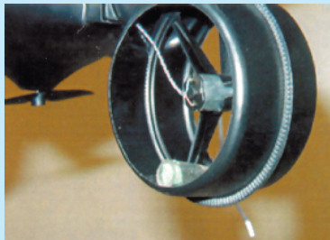
Biochemical Collector Filled by Fan Engine
