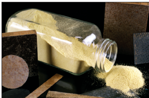
Several Products made from LaRC-LCR include films, plaques, foams, uniaxial carbon-fiber prepregs, and carbon-fiber composites.
