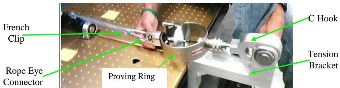
Figure 17. ARED Calibration Tool Installed for Tension Load Cells
