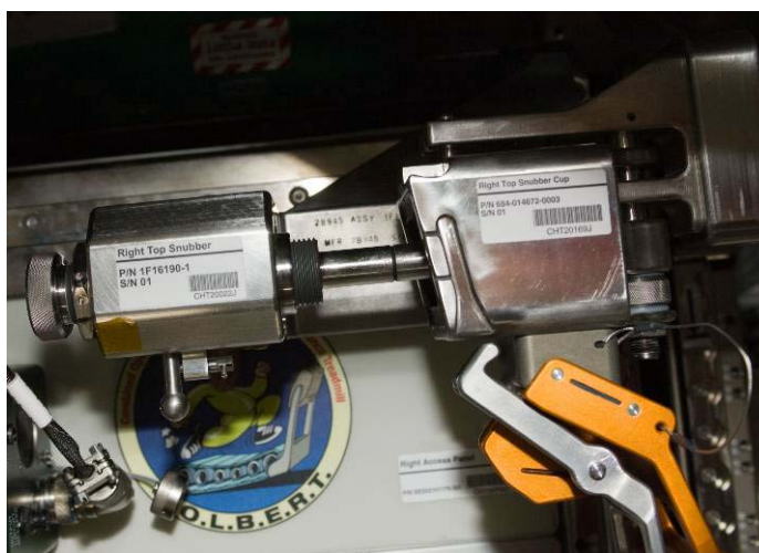
Figure 4. Snubber, Snubber Cup, and Alignment Guide Unlocked
