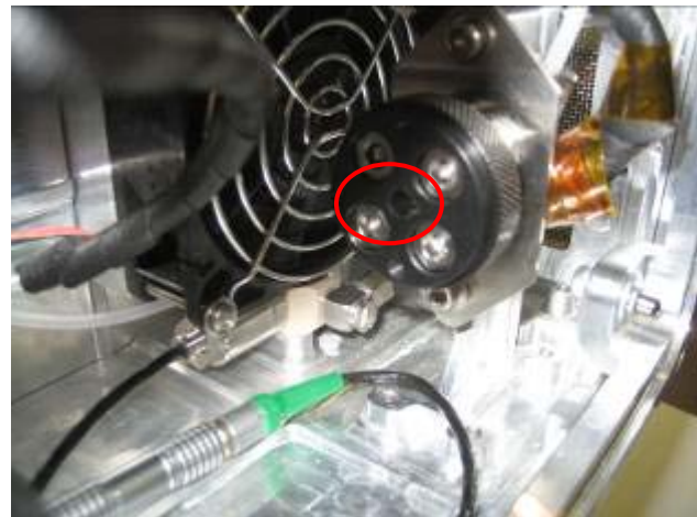
Figures 21-22. Gas Liquid Separator, Location to be Installed
