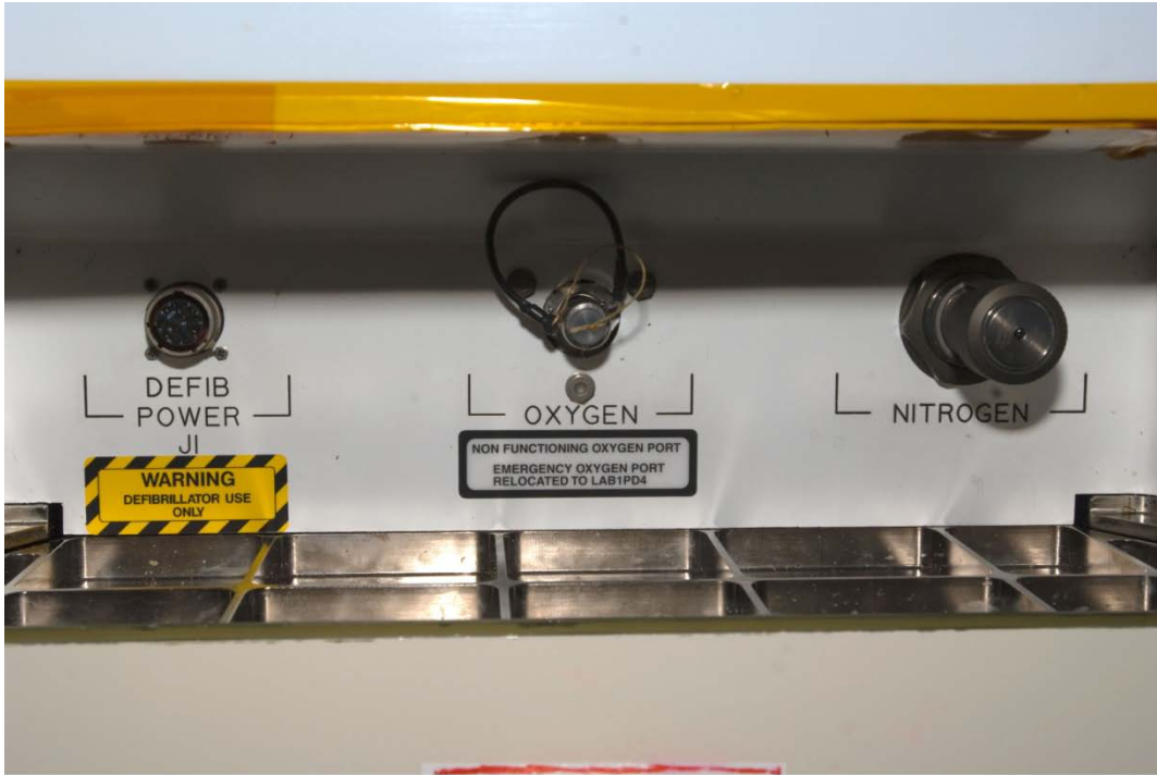
Figure 7. LAB1S4_H1: CHeCS Utility Panel With Non-Functional Oxygen Port Label
