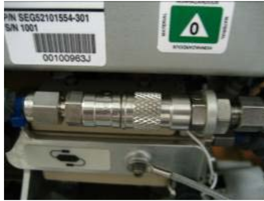
Figures 28-29. Incorrect and Correct QD Connections, Respectively
