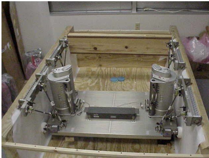
Figure 1. RED Assembled in Wooden Node 1 Mock-up
