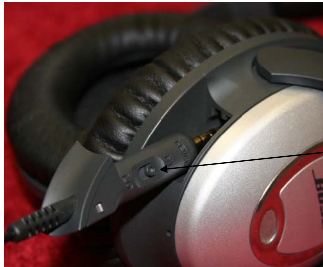
Figure 3 - Hi/Lo Switch on Audio Cable
