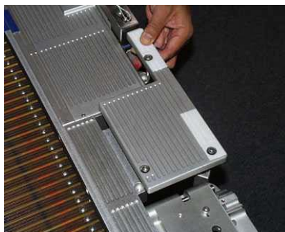
Figure 7. Aft Closeout Panel
