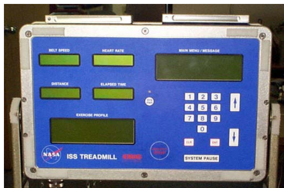
Figure 8. TVIS Control Panel
