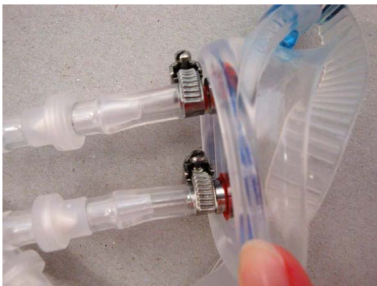
Figure 4. Hose Clamps applied to Hoses/Tubing
