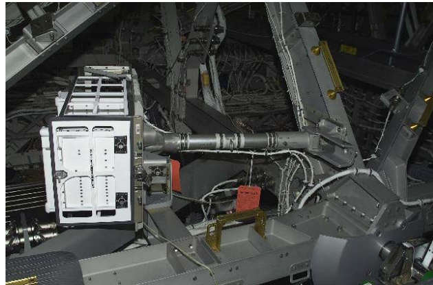
Figure 2. EVCPS attached to the S0 Truss
