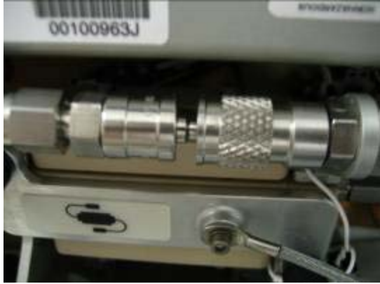
Figures 28-29. Incorrect and Correct QD Connections, Respectively
