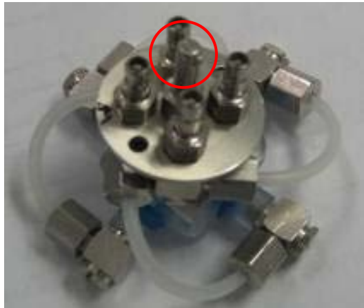
Figures 21-22. Gas Liquid Separator, Location to be Installed
