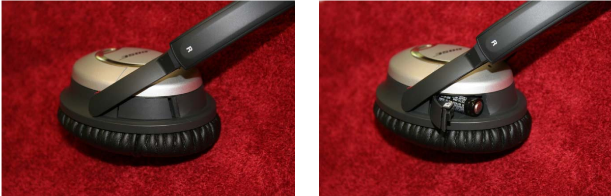
Figures 4-5. Headphone Battery Compartment (Closed and Open)
