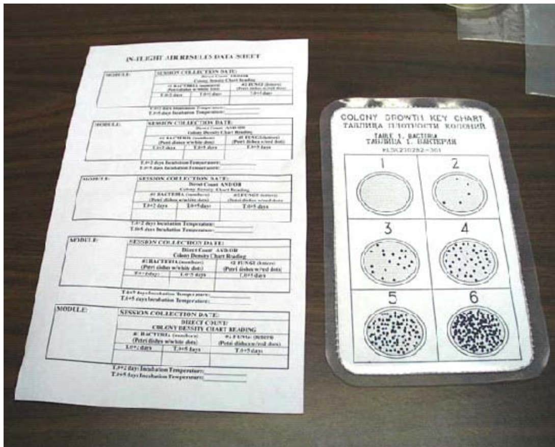
Figure 9. In-Flight Air Results Data Sheet and Colony Growth Key Chart (will not be resupplied) (Also in the procedure)
