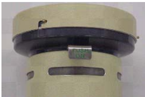
Figures 7-8. Microbial Air Sampler PUSH ON and PUSH OFF Sliding Valve (Rocker switch)
