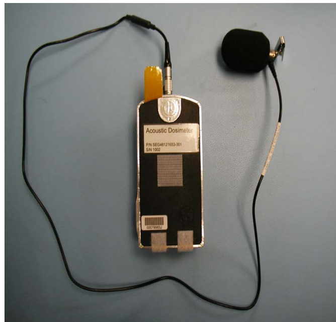
Figure 2. Protective Cover on Acoustic Dosimeter
