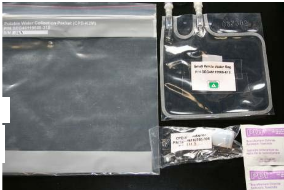
Figure 4. Contents of a Potable Water Collection Packet SRV-K (gray)
