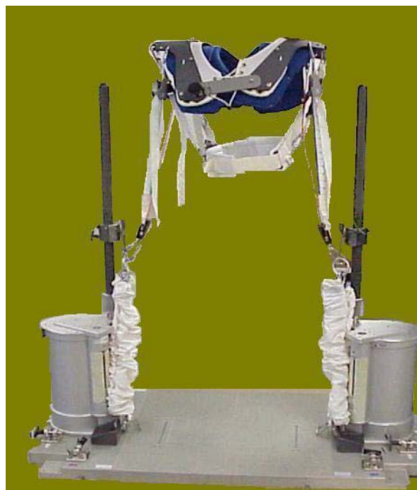
Figure 8. Example of CRES Bungees Attached to RED Assemblies
