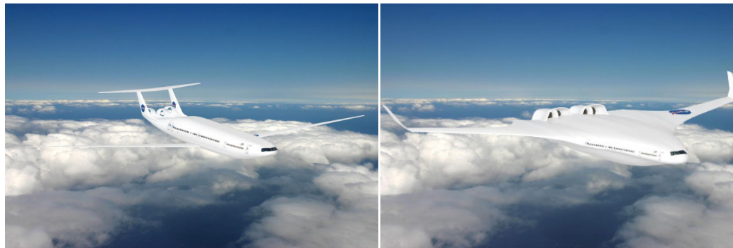
Figure 2.—MIT concepts, Double Bubble and Hybrid Wing Body, respectively.
