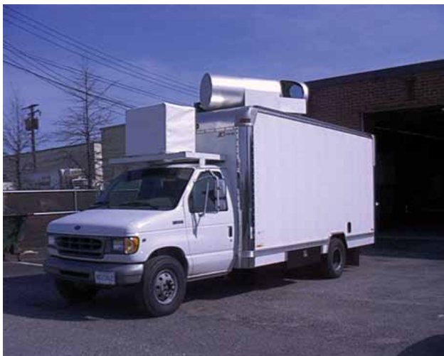
The GLOW mobile Doppler lidar measures wind profiles from surface into the stratosphere. The two-axis scanner (on the roof) allows full-sky scanning of the lidar.
