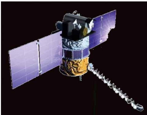
Drawing of the completed Earth-viewing Deep Space Climate Observatory (DSCOVR) Project (formerly Triana) spacecraft and instruments. EPIC awaits scheduling for launch and deployment to the Earth's Lagrange-1 point.
