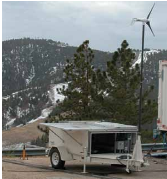
KILT was deployed at the Jet Propulsion Laboratory's (JPL) Table Mountain Facility North of Los Angeles, California. The power generating solar panels and windmill are visible in this picture.
