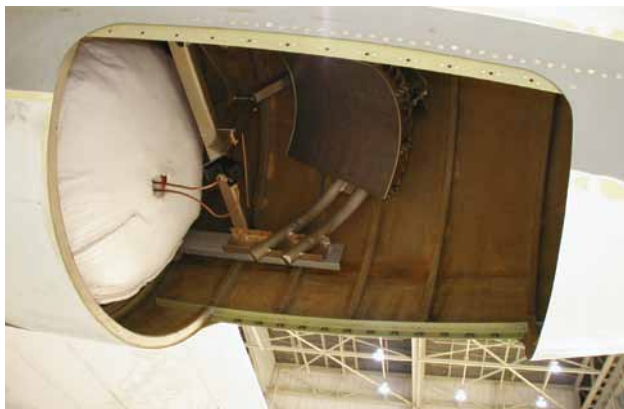
CRS instrument and antenna located in the tail section of an ER-2 SuperPod. The antenna points at nadir.
