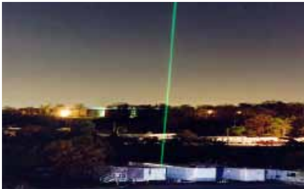
AT Lidar operating at GSFC; 532 nm beam is clearly visible.
