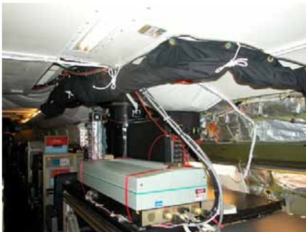
AROTAL in a DC-8 with an up-looking telescope (the black cylinder) and one laser showing.
