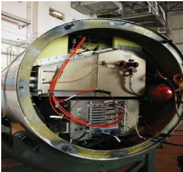
Aft view of EDOP nose showing transmitter and data system.
