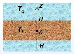
A ceramic plate of thickness 2H at  $T = T_i$  is immersed in media at  $T = T_o$
