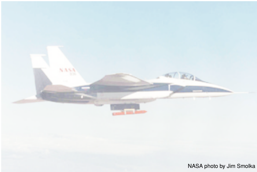
Figure 1. The PFTF Holds the Test Article underneath the F-15B airplane during flight.
