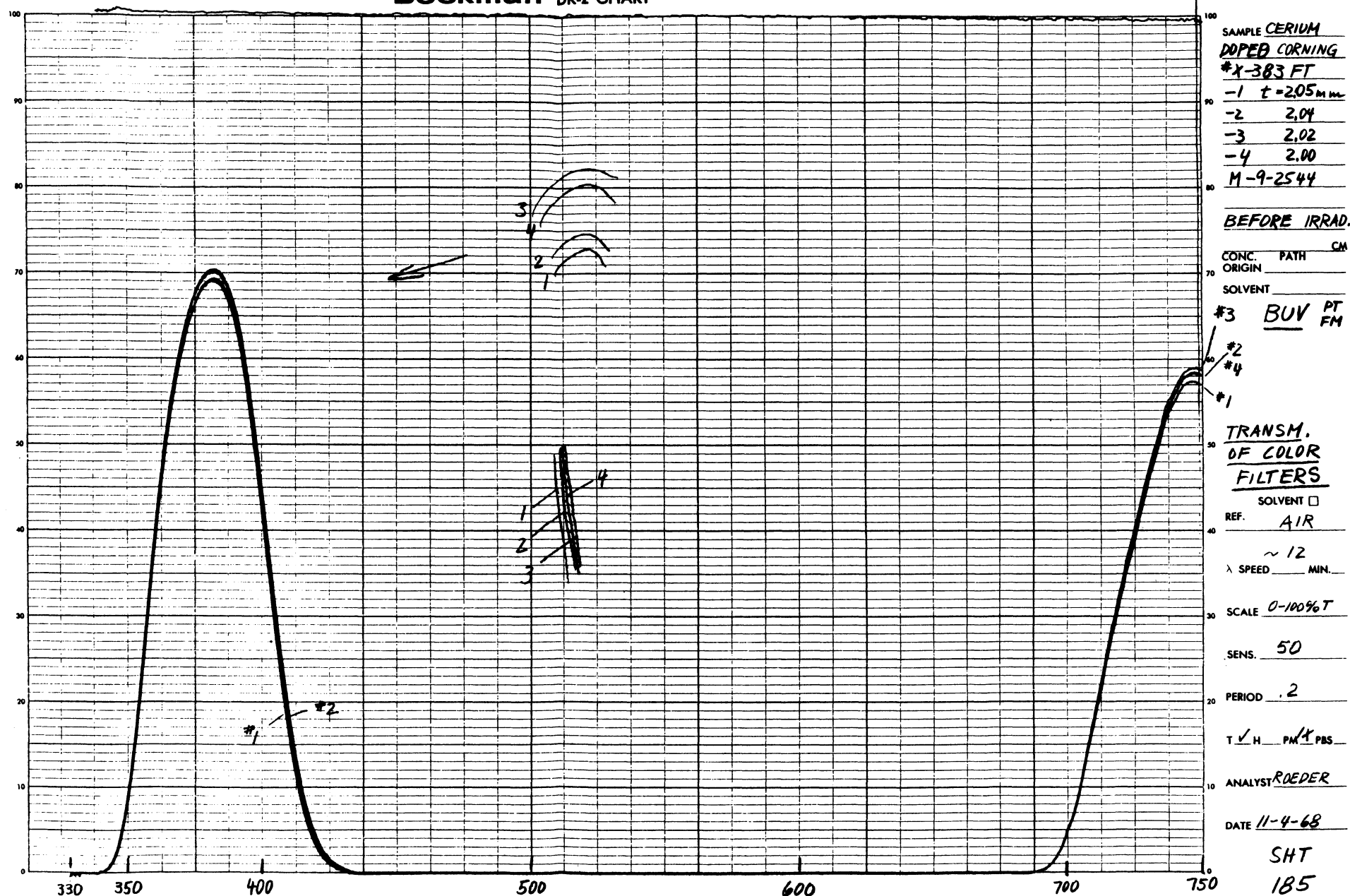
Figure 3-68. Percent Transmission of Cerium Doped Corning Filters (Before Irradiation) (2 of 2)
