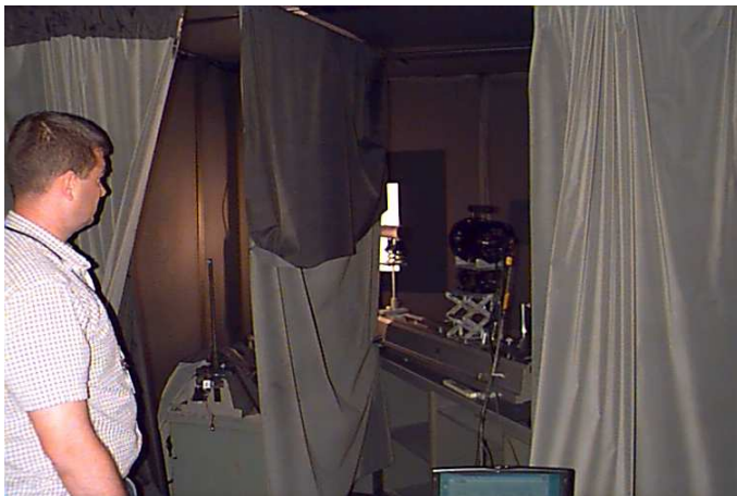
Figure 3.2: This picture shows the setup at Wallops. An Oriel lamp (obscured by curtains in this picture) illuminates a Spectralon plaque (in the center of the picture, partly obscured by curtains). A radiometer is placed on the right hand side, viewing the plaque at an angle of 45°. The curtains on the right separate the area with the radiometer from the control area where PCs and other light emitting equipment can be placed. The whole area is surrounded by black painted wooden walls that prevent light from the outside entering the area.
