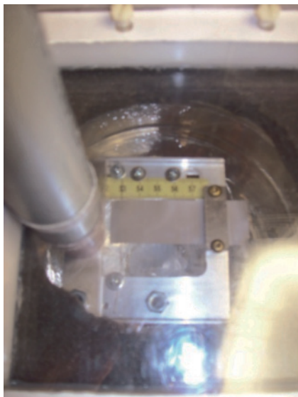
Figure 66. Sample holder with screen sample immersed in LN 2 .
