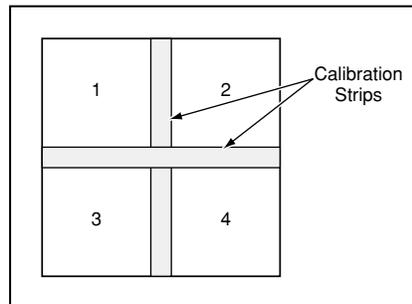
In this **Simplified Example of a Biomolecular-Signature Detector** with self-calibration, the APS array would be divided into four pixels or groups of pixels, each coated with a different substance that would act as a receptor for one of four fluorophores associated with one of four molecules that one seeks to detect.
