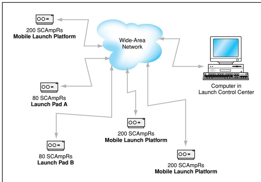
**Data Would Be Recorded Temporarily by the SCAMP-Rs** and later transmitted to the computer in the launch control center via the wide-area network. This arrangement is less complex than is that of the present system, in which the data are transmitted to redundant recording equipment via a redundant and more complex system of communication links and interfaces.
