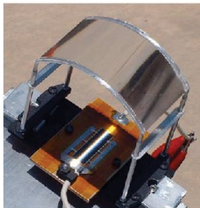
Figure 8.—The Stretched-Lens Array (SLA) focusing incident light onto PV collector.
