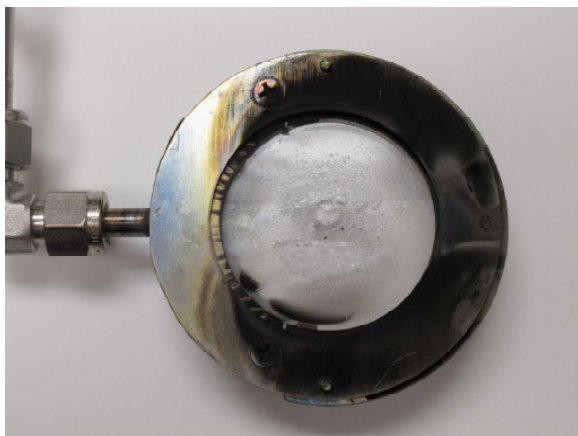
Figure 21.—Damage to a protective quartz window due to accumulated silica vapor.
