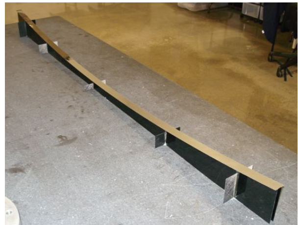
Figure 12.—Implementation of Fresnel mirror on composite rib, and assembled on a positioning tool using a frame that fixed the mirror strip position.
