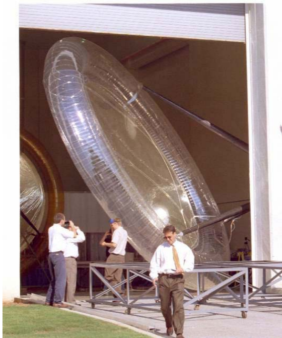
Figure 23.—Flexible 4 m by 6 m offset parabolic concentrator.
