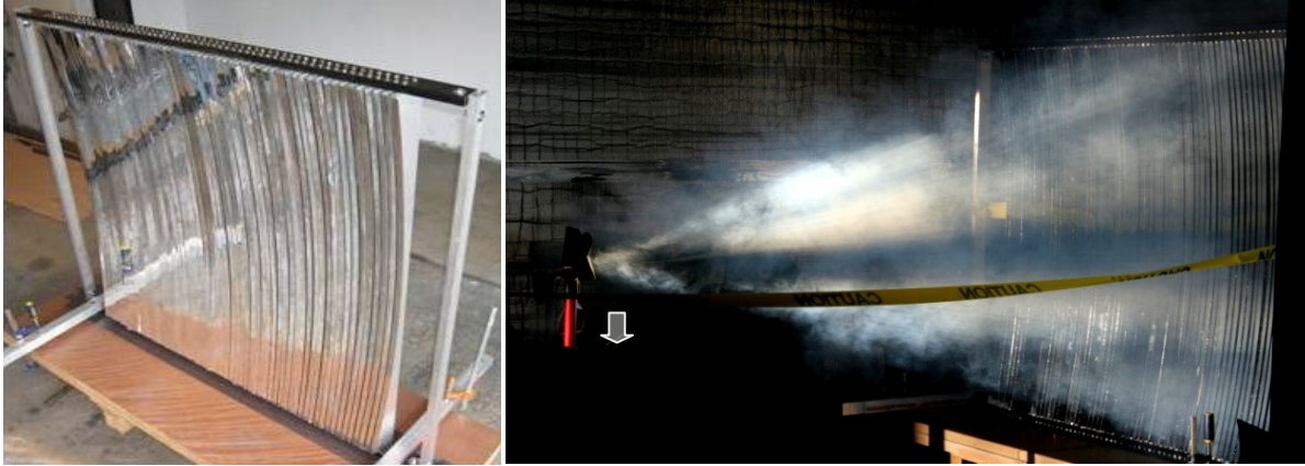
Figure 13.—Mirror test article and illumination testing using fog machine for visual feedback.
