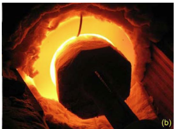
Figure 28.—(a) Demonstration heat pipe-test set up and (b) heat pipe demonstration operating at 1325 K using a Kanthal Heating Element.
