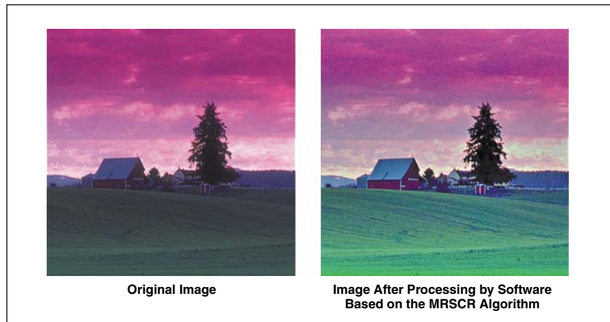
Details in Shadows are more readily perceptible after processing by software based on the MSRCR algorithm.
