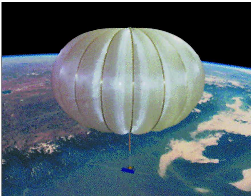
This Pumpkin Balloon weighs less than a spherical balloon of equal payload capacity. The corresponding meshed pumpkin balloon would have only a fraction of the weight of a pumpkin balloon.
