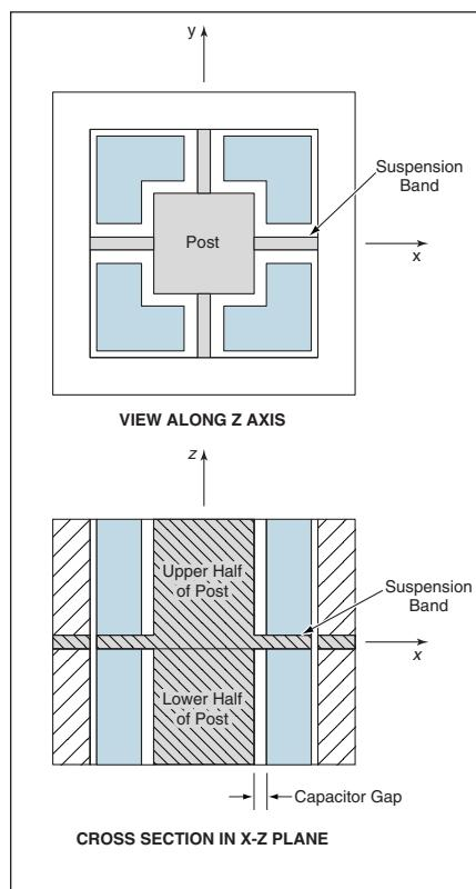
**The Outer Ends of the Post Oscillate** in the  $x$ - $y$  plane as the suspension bands flex and bend. The oscillations are affected by rotation of the entire device about the  $z$  axis.
