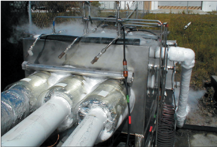
Thermal Guard Boxes at the ends of a pipe under test are used to make the fluid connections to the pipe. In addition, a temperature control device imposes a specified temperature on the outer surface of the pipe insulation.
