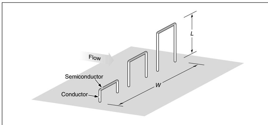
**Nanoscale Hot-Wire Probes** would be used to characterize a flow at several distances from a surface, typically ranging from tens of nanometers to a few micrometers. The lateral dimension,  $W$ , of the array of probes would be made much less than the expected characteristic dimension of lateral nonuniformity of the flow. The distance from the surface ( $L$ ) of the most distant probe would be made much less than the expected thickness of the boundary layer of the flow.
