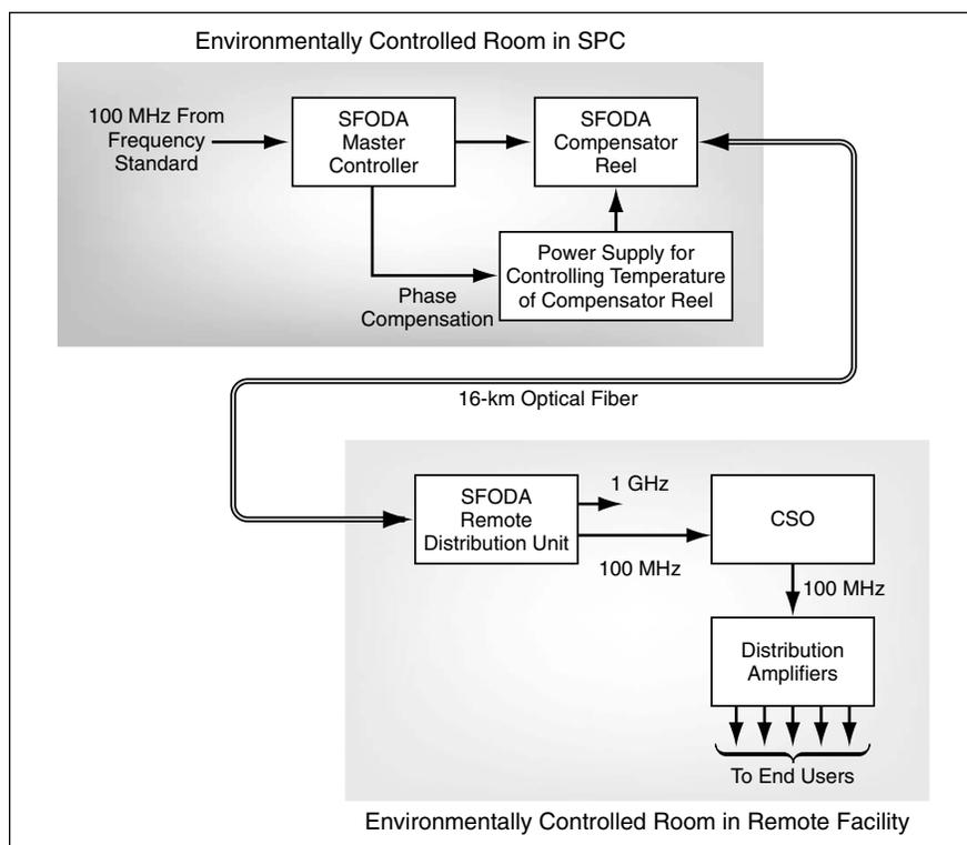
**A Frequency-Standard Signal** is transmitted over a long fiber-optic link augmented with equipment at both ends that stabilizes the output frequency and phase to a high degree.
