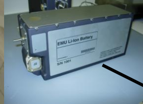
Long Life Battery (LLB) for EMU Lithium ion (Li-ion)
