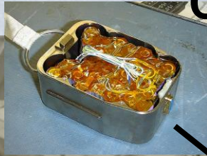
Pistol Grip Tool (PGT) Battery Nickel Metal Hydride (NiMH)
