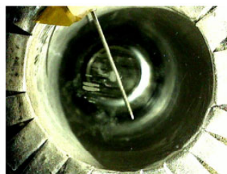
Figure 2: JSC1A simulant is transferred to chamber wall after collection experiment
