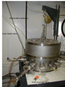
Figure 4: Vacuum chamber with interior CO 2 pressure chamber.
