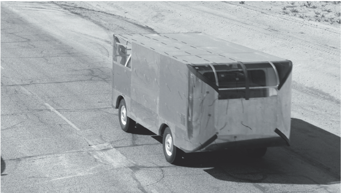
As the tufts of yarn make clear, applying a radius to all corners of the Shoebox, front and back, smoothes airflow.
