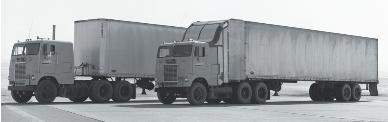
The Bat Truck, right, alongside an almost identical test truck that served as the baseline vehicle. Both tractor-trailer units were sent on multiple trips around a 312-mile loop of highways to evaluate modifications made to the Bat Truck.
