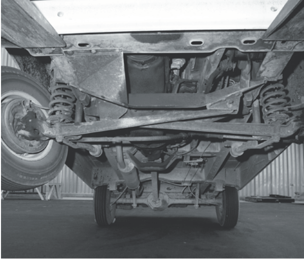
The image at left shows the underbody of the Shoebox in its stock configuration. The image at right shows the same underside after it had been sealed. This modification alone, including sealing the wheel wells, reduced aerodynamic drag by 15 percent.
