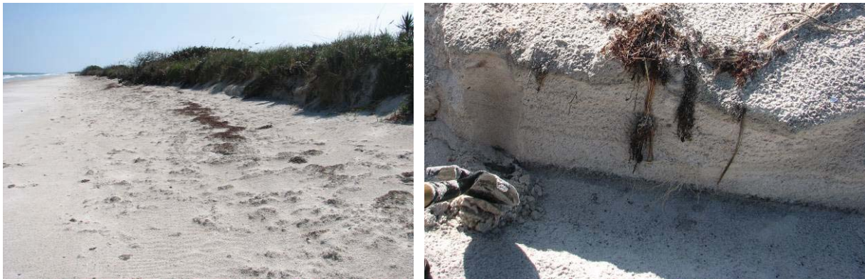
Figure 4-3: KSC LDD Sand sampling site (left). Uniformity with depth apparent (right).
