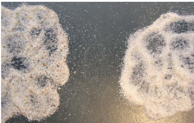
Figure 6-1: KSC LDD (left) and Mason Sand (right) visual comparison. Note the shell fragments in the KSC LDD sand.
