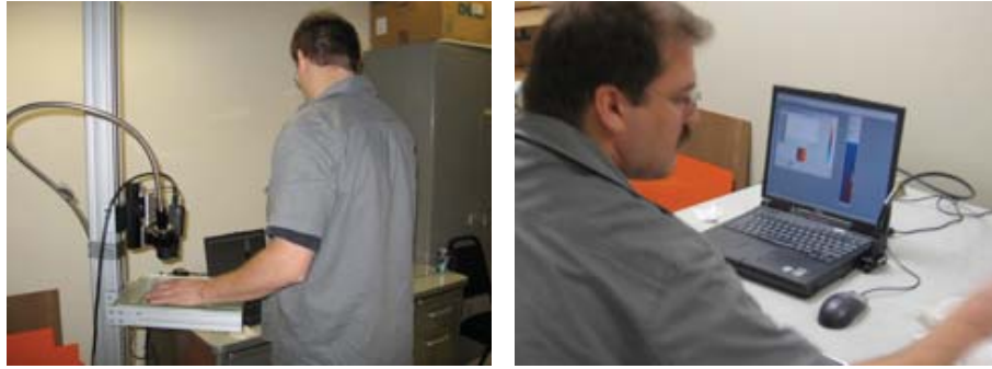
Figure 7. Engineer imaging and measuring PER at a damage site. A commercially available GFP with special software was used for these measurements.
