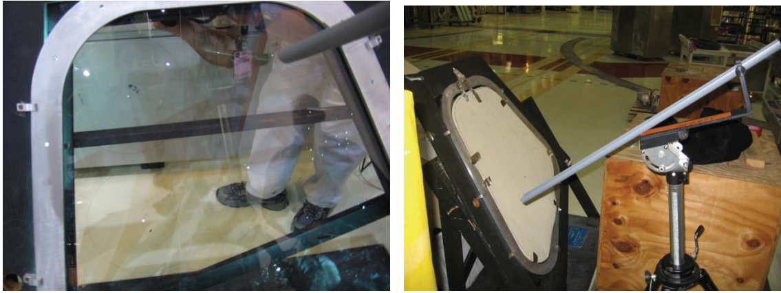
Figure 5. Experimental arrangement set-up for inflicting bruise damage on glass panes.
