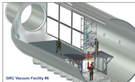
Figure 1.—TDU test layout with the Core Simulator, NaK heat transport components, and Stirling PCU in the vertical truss and the Six HRS radiators supported by the central monorail.
