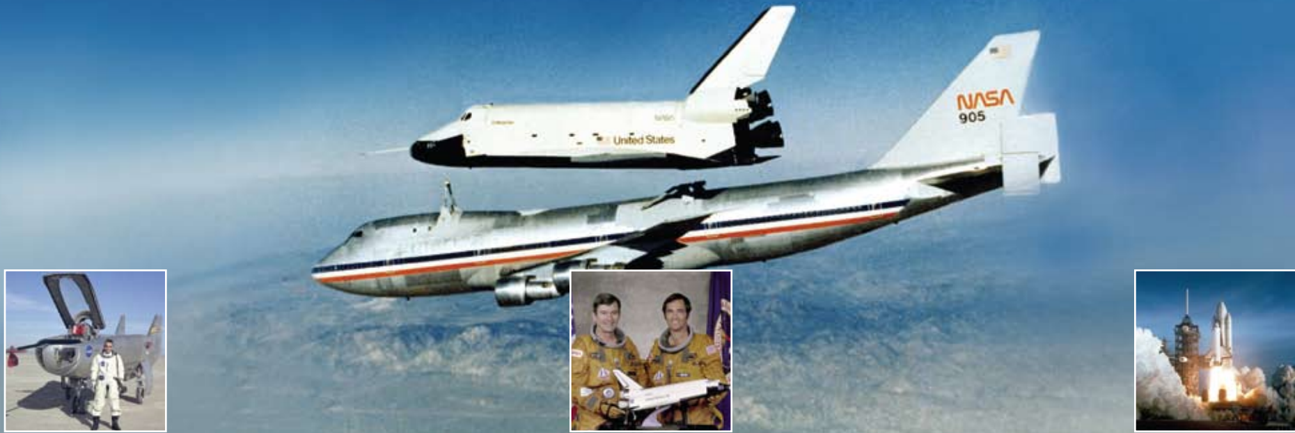
The Space Shuttle prototype Enterprise rises from NASA's 747 Shuttle Carrier Aircraft to begin a powerless glide flight back to Dryden Flight Research Center. The Enterprise test flights verified the aerodynamic and control characteristics of the orbiters in preparation for the first space mission with the orbiter Columbia. Inset images (left to right): The M2-F3 aircraft, part of NASA's lifting body program, contributed to the database that led to the development of the Space Shuttle Program; STS-1 crewmembers John Young and Robert Crippen; the launch of STS-1 in April 1981.
