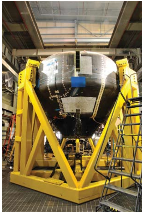
The Composite Crew Module allows NASA researchers to test materials and methods that may one day be applied to spacecraft constructed using composite materials.
