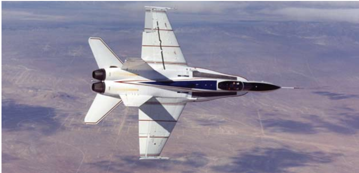
Dryden Flight Research Center's Active Aeroelastic Wing aircraft shows off its form during a research flight.
