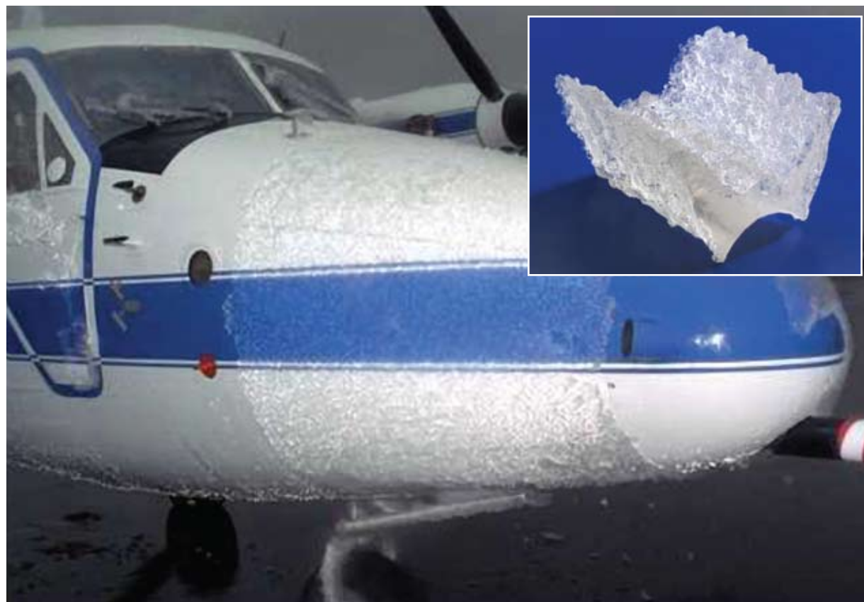
Supercooled large droplet conditions caused the buildup of ice on this aircraft. Using the NASA LEWICE software, aircraft manufacturers can model the ice accretion and the various shapes the ice can form (such as the inset example) on aircraft surfaces.
