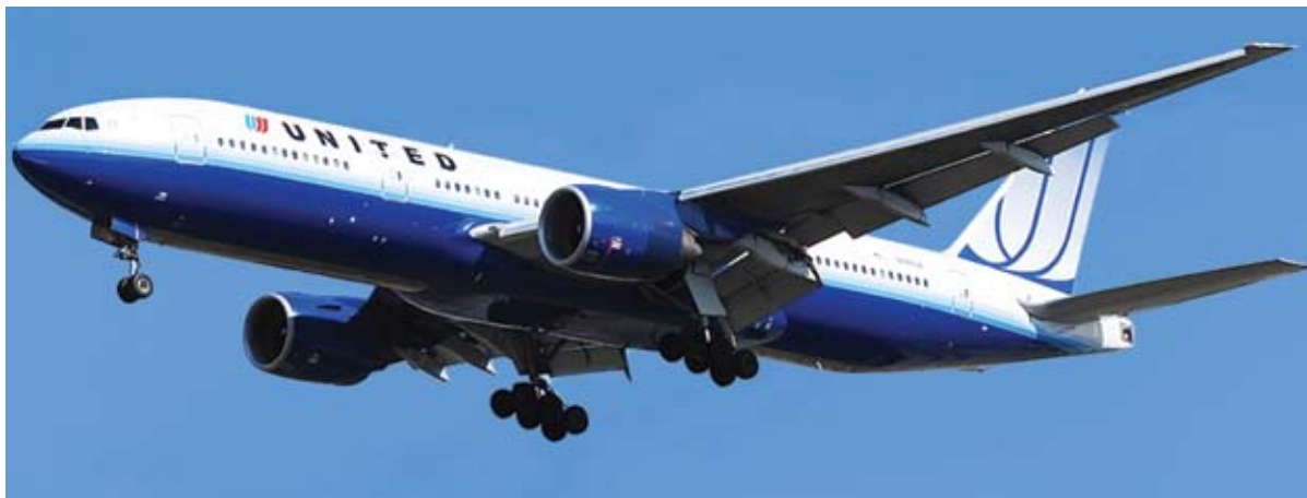
In 1994, the Boeing 777 became the second commercial airliner to fly using DFBW. For commercial aircraft, the replacement of heavy mechanical systems with DFBW controls provides greater fuel efficiency or the ability to carry more passengers or cargo.
