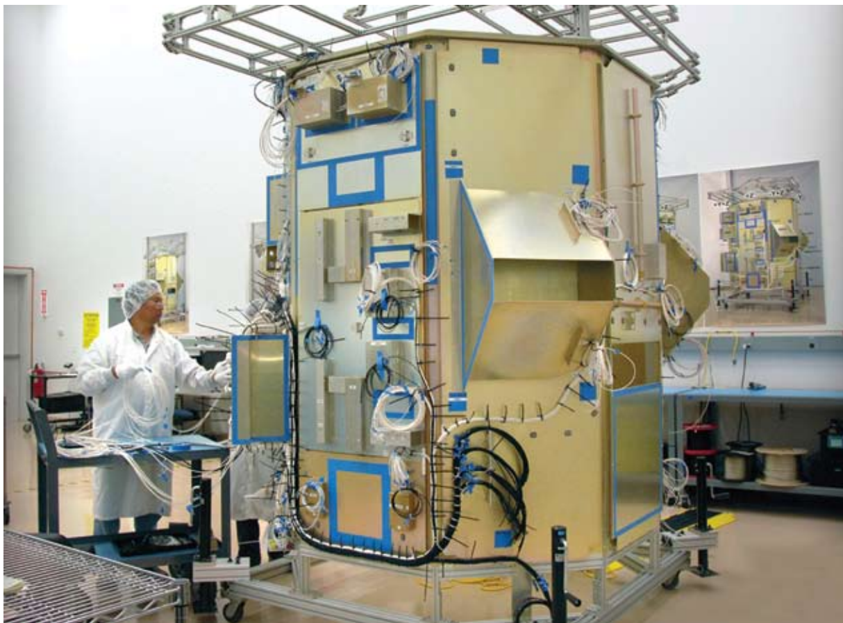
This mock-up of the Landsat Data Continuity Mission is essentially a full scale model of the actual satellite, which is scheduled for launch in 2012. The mock-up enables engineers to check that all components seat and connect correctly.
