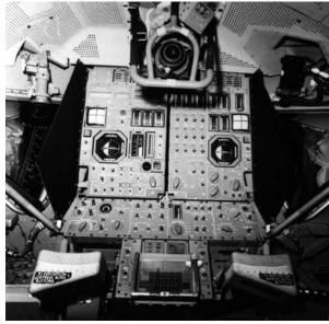
The Primary Guidance, Navigation, and Control System of the Apollo Lunar Module. The display and keyboard (DSKY, pronounced "diskey") interface used by the astronauts to input commands can be seen in the bottom center of the image.
